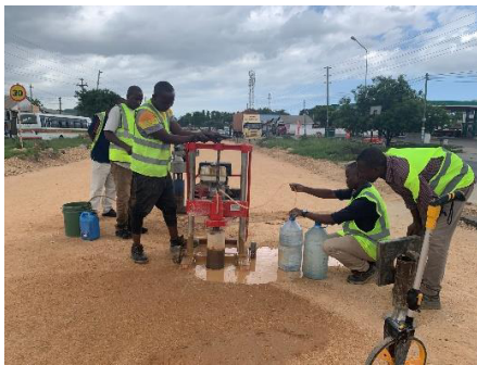
Photo No. 3: Coring test on C1 Pavement
