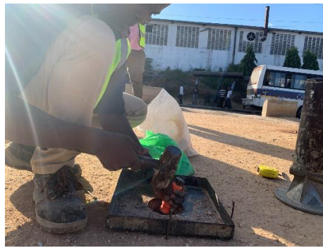
Photo No. 4: Field Density test on C1
