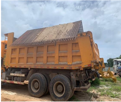
Sieve truck for natural sand as seen on contractor's camp site.
