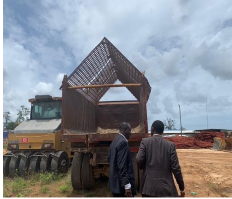
Sieve truck for C1 materials as seen on contractor's camp site.
