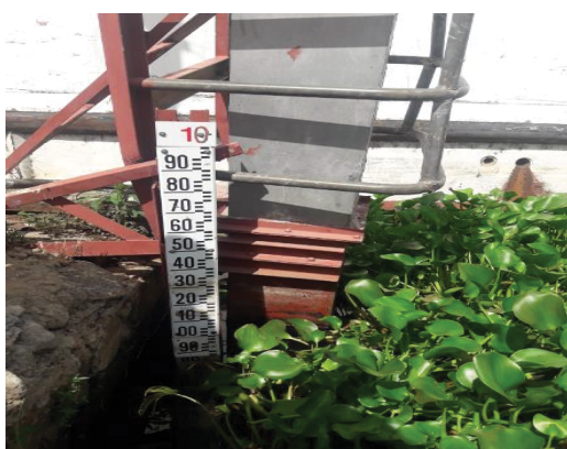
Figure 3.3(a): Manually operated water-level recorder for measuring water level located at Lake Victoria.
