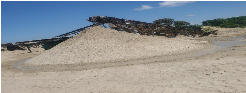
Photo 11. 4: Special equipment to wash/clean sand from deleterious materials for BRT Phase 3. The Photo was taken by Auditors at Buza Contractor’s Campsite on 29 November 2024
