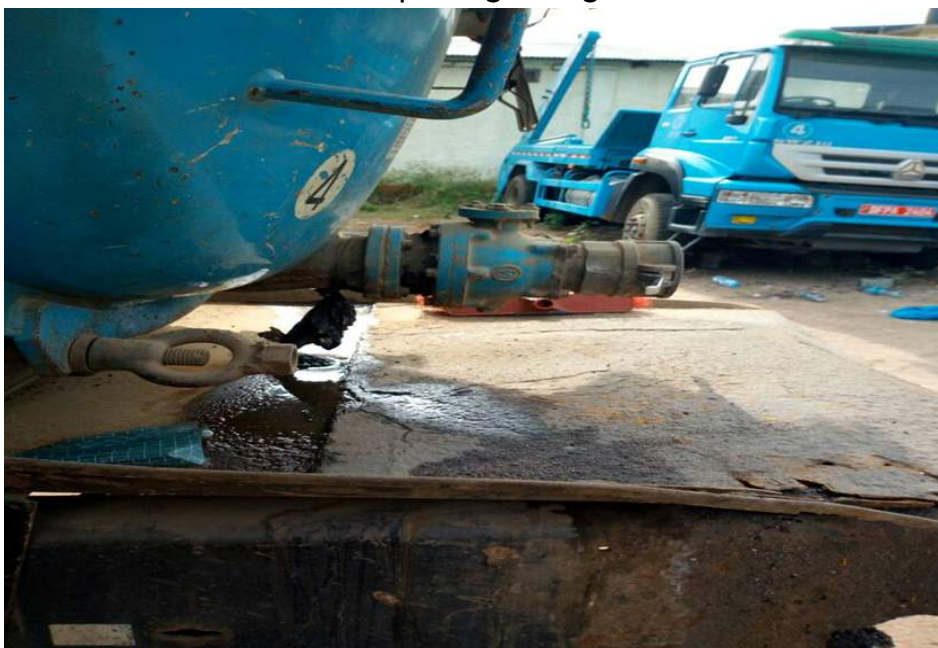
Photo 4.5 (b): Showing the dilapidated emptying trucks that do not meet standard for transporting sewage
