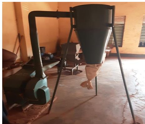
Photo 3.4(b): Cassava milling machine operated by Diesel engine as developed by SIDO-Kigoma. Photo taken at MWISCBITA women on 7 th October, 2022.
