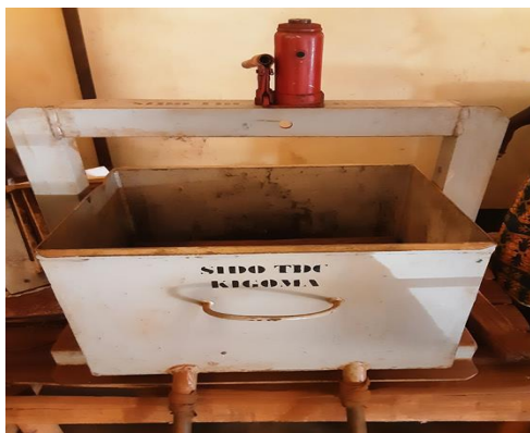
Photo 3.4(a): Starch extraction machine which is manually operated by using hand jerk to press 30 stacks of cassava per week. Photo taken at MWISCBITA Women as taken by Auditors on 7 th October, 2022.
