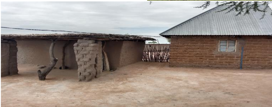
Photo 3.7: Cable close to ground and easily reachable. Photo taken on 29 th December, 2022 at Negezi village Kishapu
