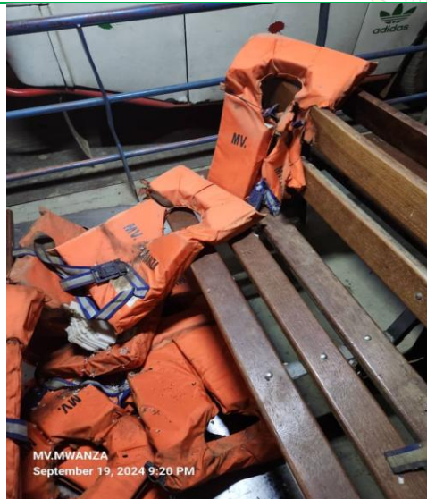
Photo 3.7(c) Defective Life jacket equipped on MV Mwanza.
