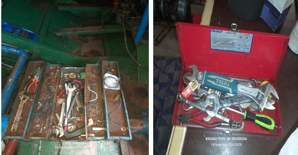
Photo 3.3: Mechanical Toolbox with Insufficient Maintenance Tools (September 2024)
