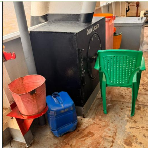
Photo 3.5(c): Fire bucket without dry sand as observed in MV Kilindoni on 17 September 2024.
