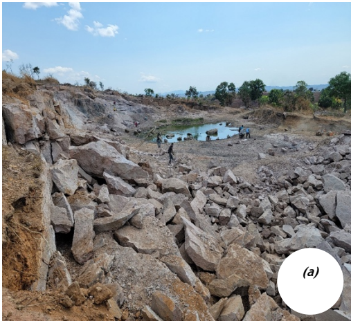
Photos 3.3 (a & b): Open Pits without Embankments to act as a stopper of falling rocks (Photos Taken by the Auditors During a Site Visit in Ruvuma Region on 22 nd September 2023)
