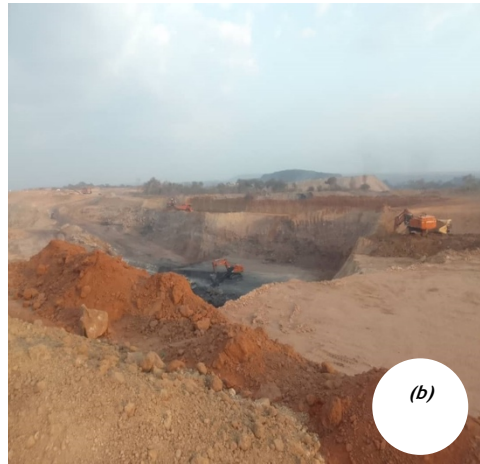
Photos 3.3 (a & b): Open Pits without Embankments to act as a stopper of falling rocks (Photos Taken by the Auditors During a Site Visit in Ruvuma Region on 22 nd September 2023)
