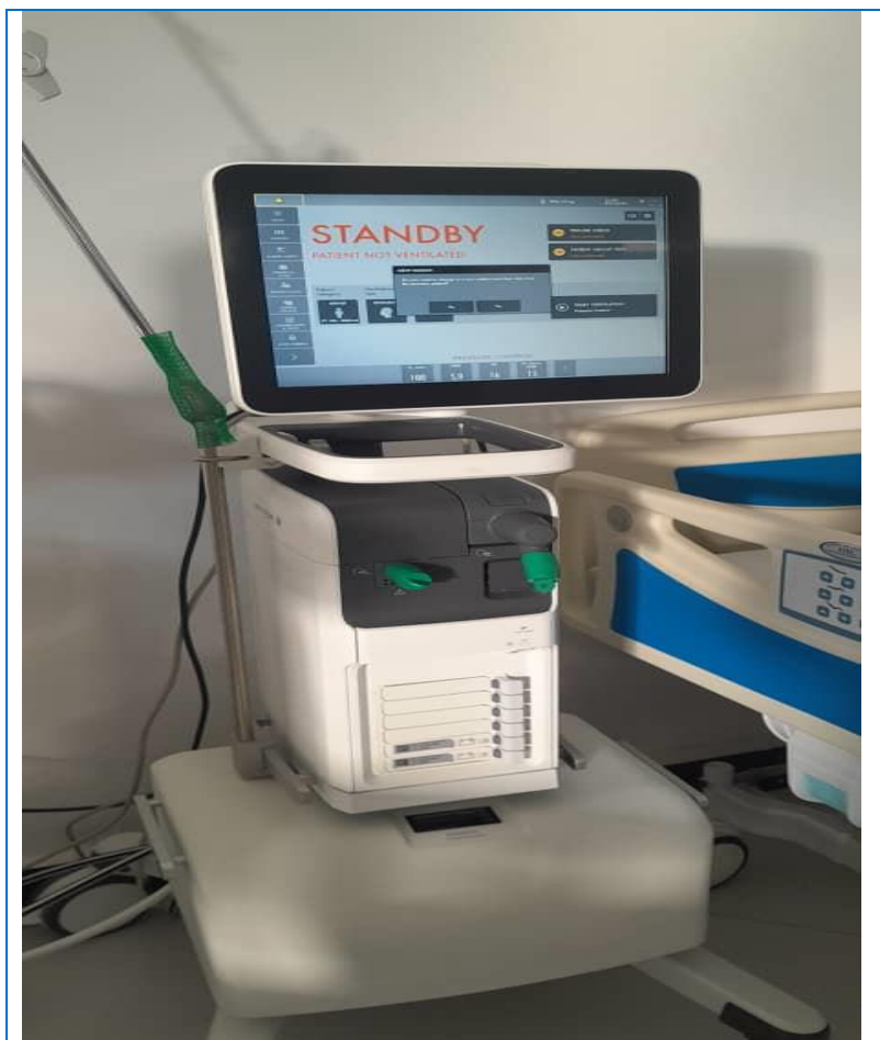
Photo 01: Ventilator (Adult and Pediatric) at ICU Unit not operational because of high operational demand of oxygen purity level at 96%
